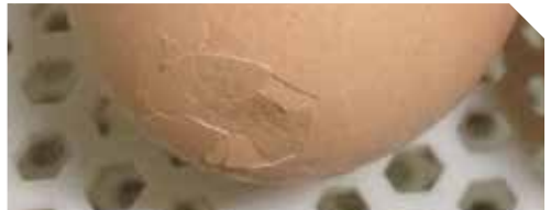
Excessive vacuum pressure on the egg lifter has caused damage to the blunt end of the egg.
