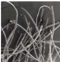
A sample of 'trimmed' wool with individual fibres shown clearly cut.
