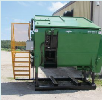
The Green Machine is a slow rotating horizontal four auger mixer that combines deadstock with wood shavings for active decomposition.
