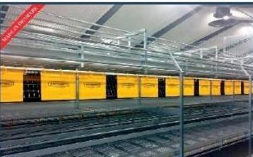
← **New** feed trough with built in step/bumper rail standard on all tiers. The ergonomic wide flat top is gentle on the feet and helps prevent damage to the egg trays.
