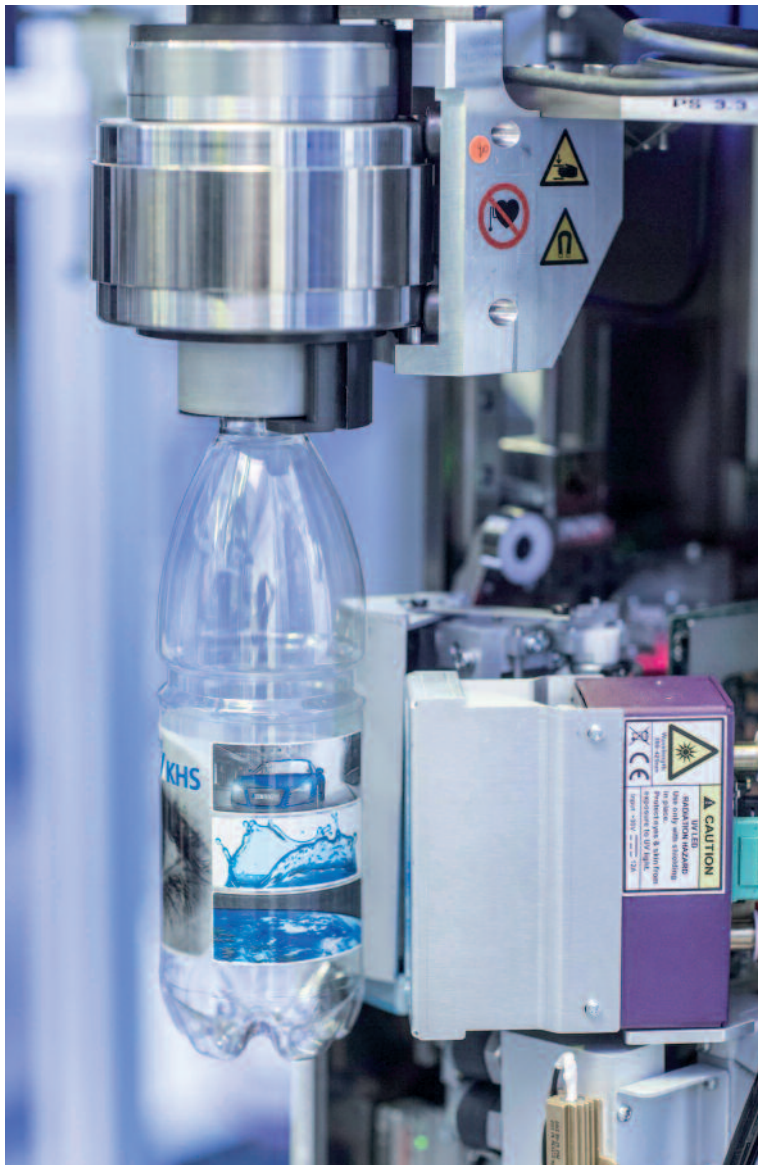
The empty PET bottles to be printed are handled by their necks on the Innoprint.
