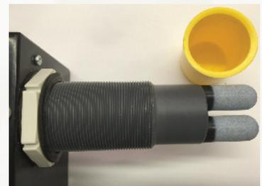
The photograph above shows typical CO<sub>2</sub> sensors in a setter, protected by sensor protection caps. If the caps become clogged with dust or condensation, the sensor will give an artificially high reading.
