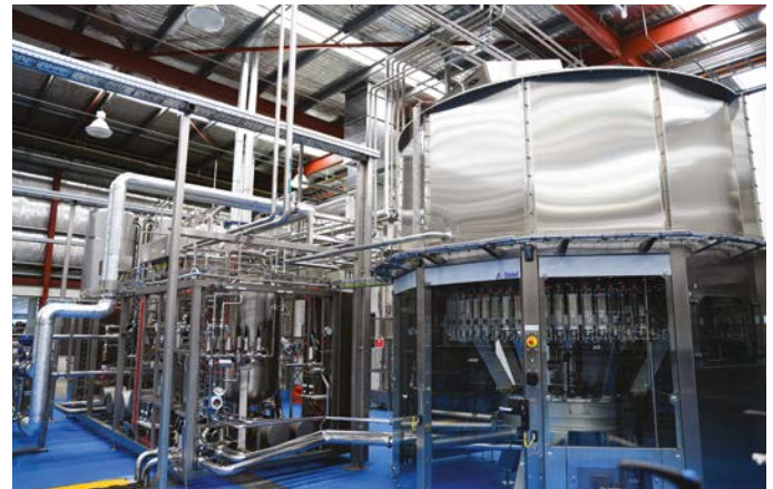
The line is running at 12,000 bph for the aseptically filled drinks and up to 18,000 bph for the CSD products (photo: Sidel)
