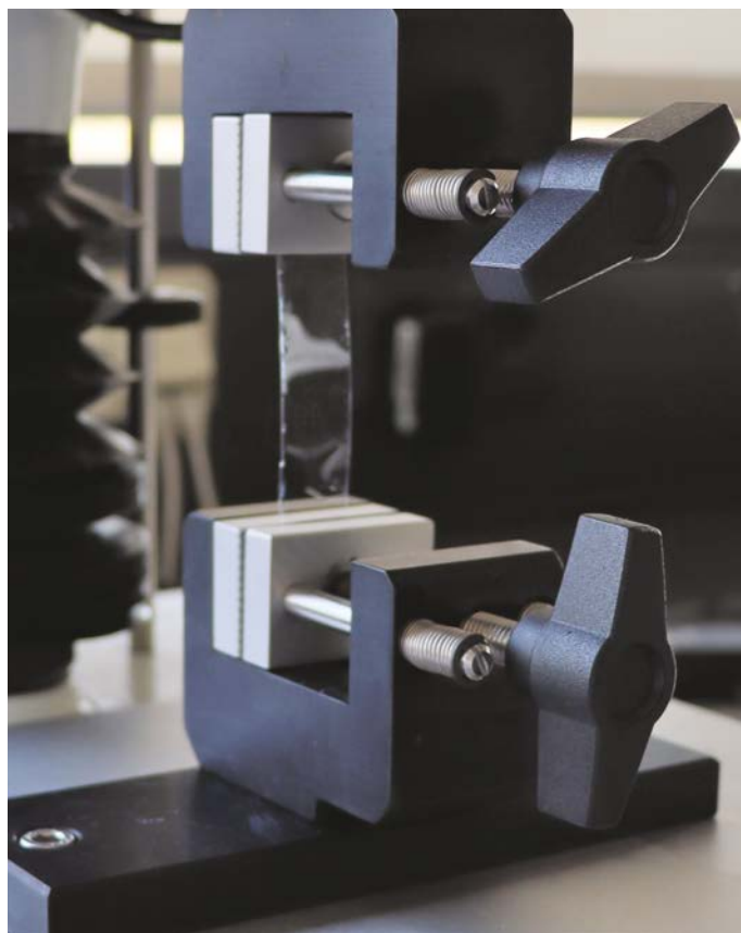
PLA film in a tensile testing device. These bio-based films will be coated with bio-based material to enhance the oxygen and water vapour barrier properties (photo: University of Albstadt-Sigmaringen)
