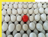
Wireless Egg Node It identifies exact locations where egg damage takes place
