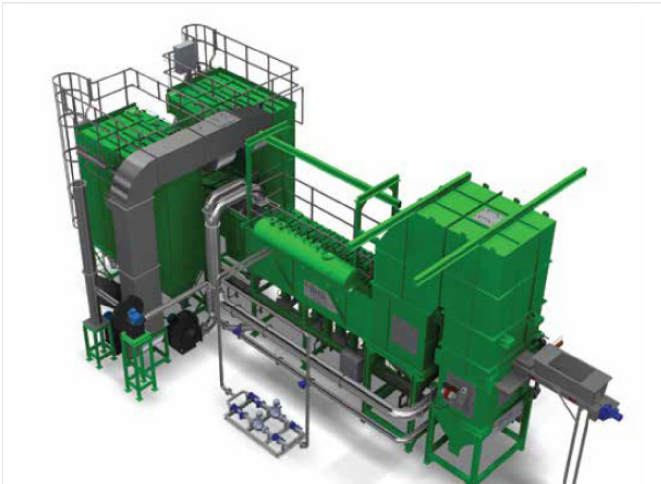
CHICKEN POWER | BHSL Hydro's Fluidised Bed Combustion System
